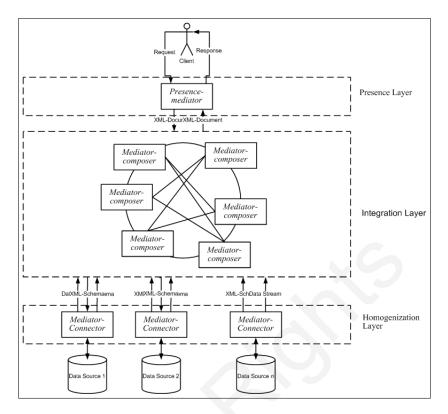
Figure 1: The Three-Layer Mediation Architecture
